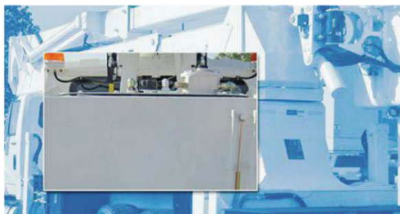
5. Reservoirs from 18 to 12 gal fabricated from aluminized steel are hot-dip-coated on both sides with an aluminum-silicon alloy to avoid the contamination problems inherent to uncoated steels.
