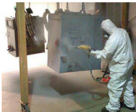
6. Tank and fill necks manufactured at The IFH Group are shown being powder-sprayed.
